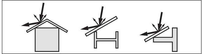
Fig. 28: Cover flat, large-area profiles with deflectors
